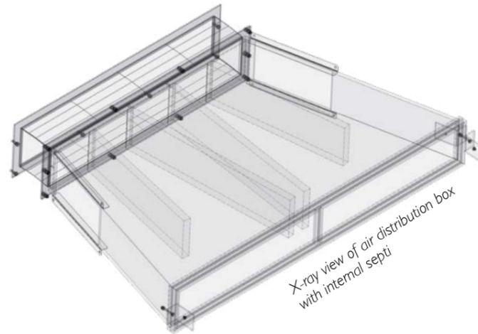
X-ray view of air distribution box with internal septa
